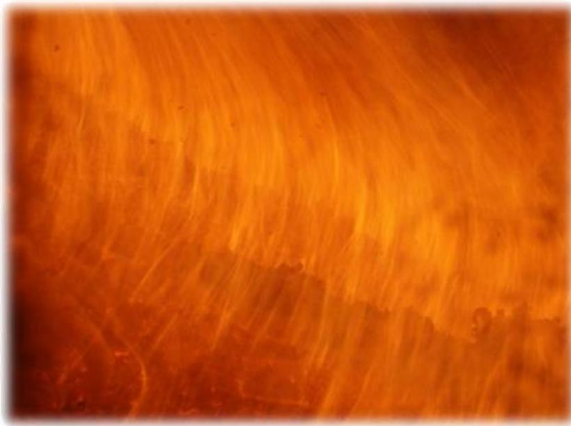
*This is a great photograph showing the streams of volatile gasses being released from the fuel and rising to the top of the chamber where the combustion process will be complete.*
